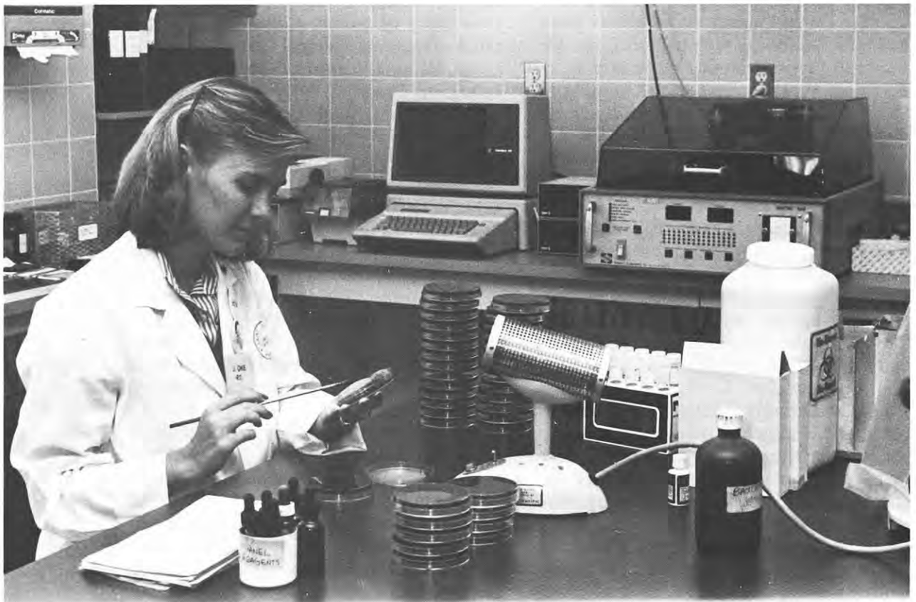
Technologist Joann Oke is performing the 'time honoured' procedure of 'streaking' a plate for isolation and identification of bacteria. In the right background is an automated sampler analyzer for detecting growth in blood cultures in as little as two hours. Previous to 1980 this would have required 96 hours. Also in the background is a computer console and display; all work operations are computerized with a terminal at each work area.
