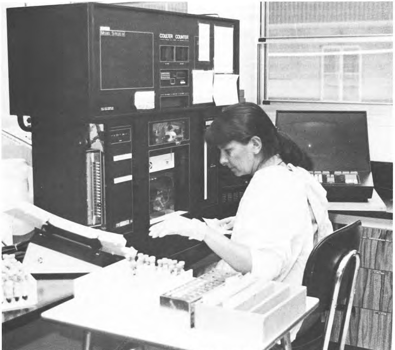
The Automatic Blood Cell Counter, operated by haematology technologist Marian Matlovich, can count and differentiate the three normal types of white cells as well as red cells and platelets plus haemoglobin concentration, all in less than one minute. There is a video display of cell characteristics and an automatic print-out of results. Twenty-five years ago this would have required at least 30 minutes.
