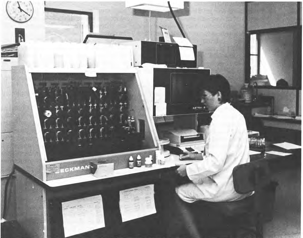
The Automated Chemical Analyzer, operated by charge technologist Joan Crosby, can determine up to nine substances in a blood sample in 30 to 60 seconds. The results are produced as a print-out as well as being monitored on a video display. These tests would have required up to four hours to perform 35 years ago. SJH Staff Photo
