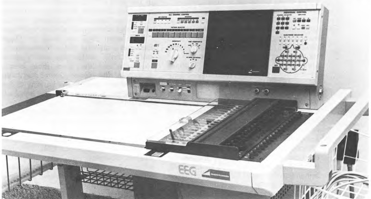
The modern EEG is readily portable; it is operator programmable with simultaneous EEG and video recording capabilities.
