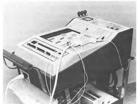
Modern Electrocardiograph, one-third the size and one-quarter of the weight of the 'pioneer' machine. SJH Staff Photo
