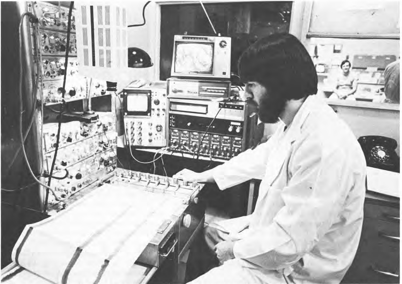
Technician Rod Kosmick at controls of electronic monitoring system developed by Dave Miller for Dr. Walters and Dr. Effer. A T.V. camera mounted over the chart allows the staff in the special obstetrical unit, seen through the window in the background, to observe the foetal and maternal heart-rate. At the same time the technician can observe any unusual actions of the patient on his T.V. monitor.
